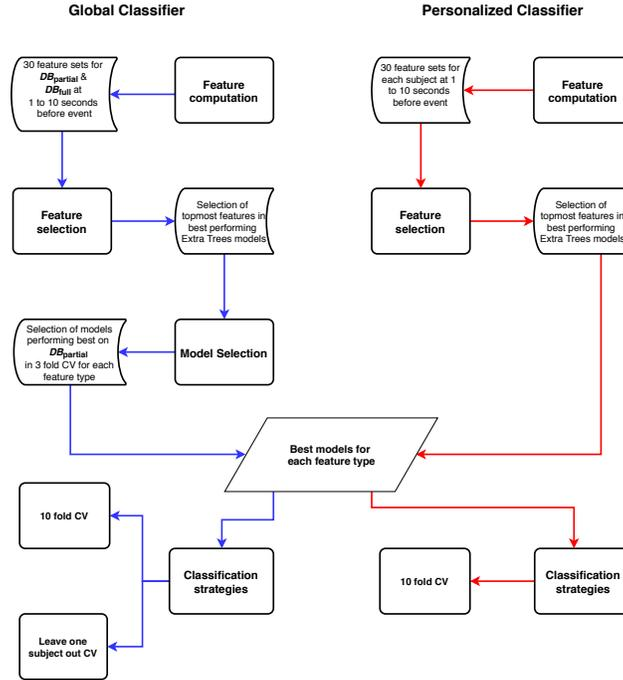
**Figure 2.** Flowchart of the complete classification approach. Blue arrows mark the flow for global classifiers, red arrows represent the personalized classifiers.
